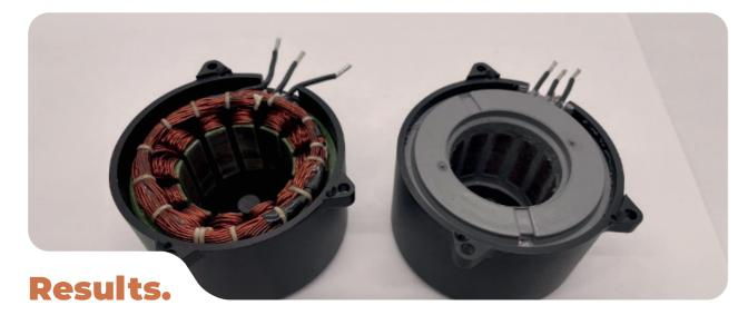
The following charts show, that the thermal performance of the Keramold<sup>®</sup> 20 was better than the potted option, and of course way better than the bare option. In that case study, the molding process was not optimized due to cost reasons. This leads to the assumption, that the thermal performance can be still improved which will even further increase the difference to the potted material.
